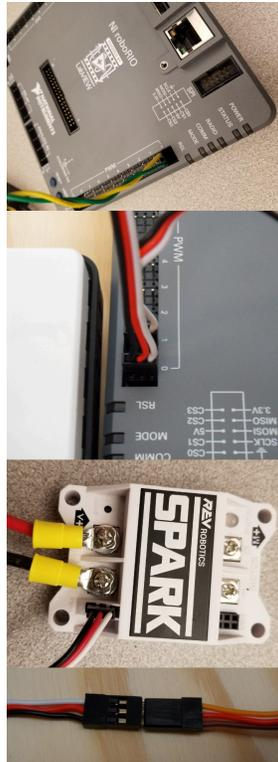
Requires: 4x PWM cables (if using non-integrated wire controllers), 2x PWM Y-cable (Optional)
