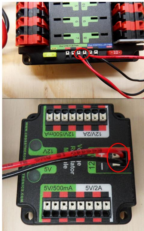
Requires: Wire stripper, small flat screwdriver (optional), 18AWG red and black wire
