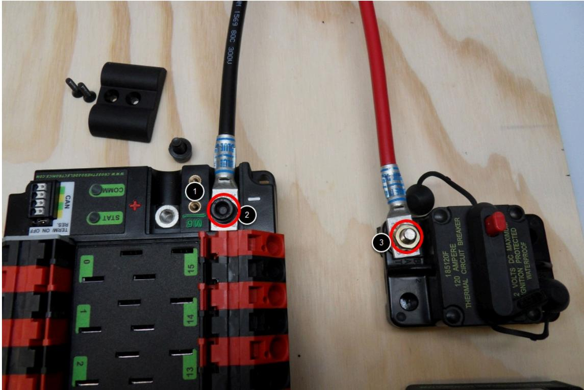
Requires: Battery Connector, 6AWG terminal lugs, 1/16" Allen, 5mm Allen, 7/16" Box end
