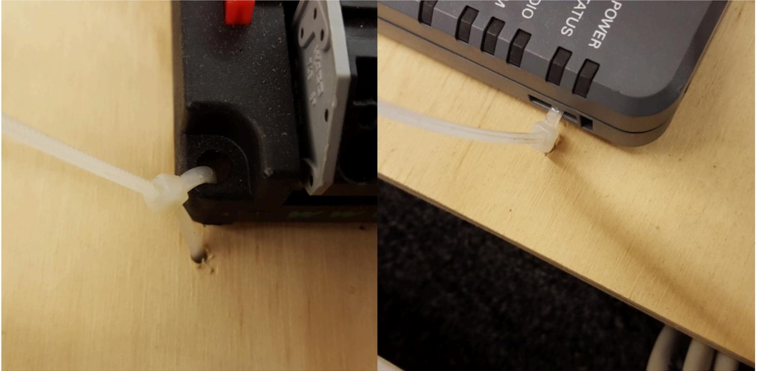
Using the Dual Lock or hardware, fasten all components to the board. Note that in many FRC games robot-to-robot contact may be substantial and Dual Lock alone is unlikely to stand up as a fastener for many electronic components. Teams may wish to use nut and bolt fasteners or (as shown in the image above) cable ties, with or without Dual Lock to secure devices to the board.
