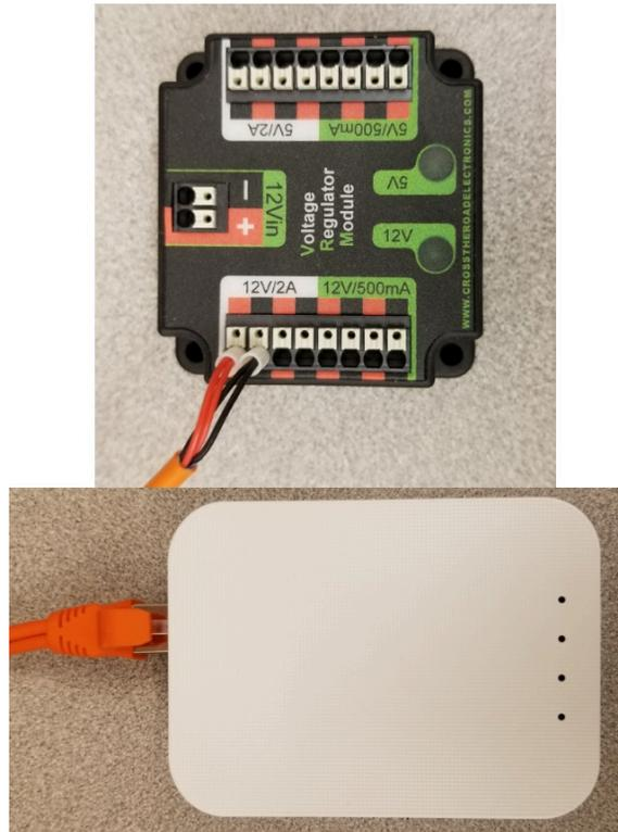
**! DO NOT connect the Rev passive POE injector cable directly to the roboRIO. The roboRIO MUST connect to the female end of the cable using an additional Ethernet cable as shown in the next step.**
