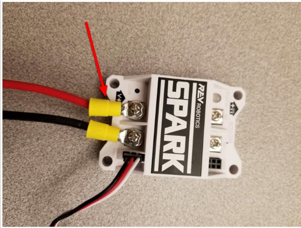
Requires: Wire Stripper, Small Flat Screwdriver, 10 or 12 AWG wire, 10 or 12 AWG fork/ring terminals (terminal controllers only), wire crimper
