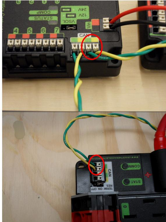
Requires: Wire stripper, small flat screwdriver (optional), yellow/green twisted CAN cable
