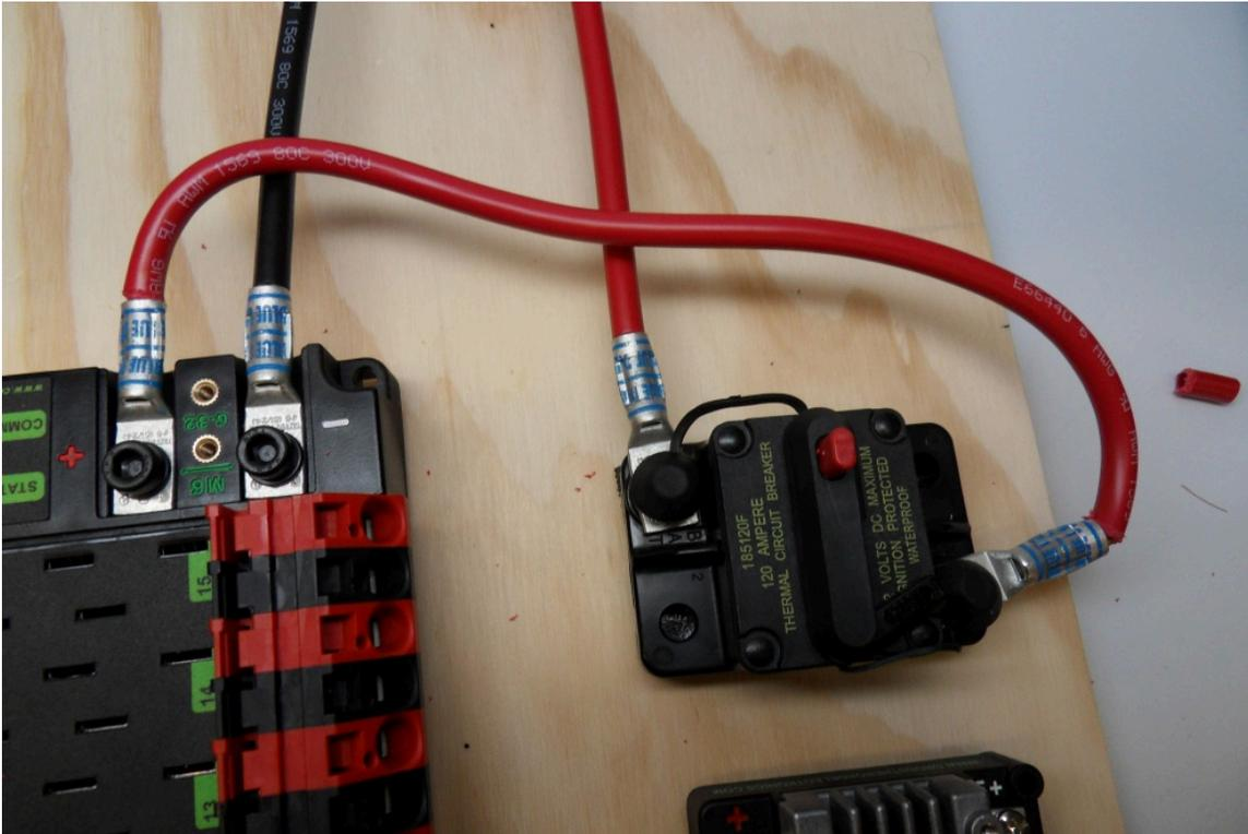
Requires: 6AWG red wire, 2x 6AWG terminal lugs, 5mm Allen, 7/16" box end
