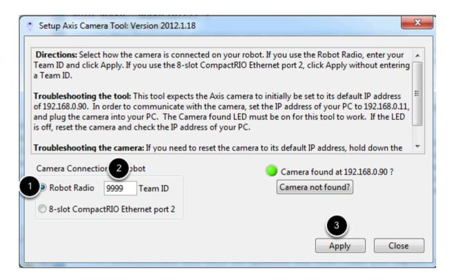
The recommended configuration (and the default expected by the robot code examples and FRC Dashboard) is to connect the camera to the Robot Radio. To configure the camera for this setup:
