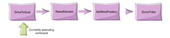
Commands let you break up the tasks of operating the robot into small chunks. Each command has an execute() method that does some work and an isFinished() method that tells if it is done. This happens on every update from the driver station or about every 20ms. Commands can be grouped together and executed sequentially, starting the next one in the group as the previous one finishes.
