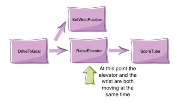
Sometimes it is desirable to have several operations happening concurrently. In the previous example you might want to set the wrist position while the elevator is moving up. In this case a command group can start a parallel command (or command group) running.
