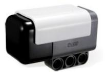
WPILib directly supports one compass, the HiTechnic Compass. This part connects to the I2C port on the Digital Sidecar. It is important to note that there is only one I2C port on each of these modules.
