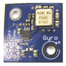
The Gyro object should be created in the constructor of the **RobotBase** derived object. When the Gyro object is used, it will go through a calibration period to measure the offset of the rate output
