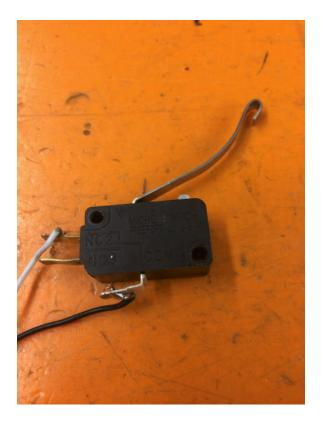
Limit switches can have "normally opened" or "normally closed" outputs. The usual way of wiring the switch is between a digital input signal connection and ground. The digital input has pull-up
