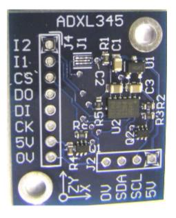
The ADXL345 is a three axis accelerometer provided as part of the sensor board in the 2012-2014 KOP. The ADXL345 is capable of measuring accelerations up to +/- 16g and communicates over I2C or SPI. Wiring instructions for either protocol can be found in the FRC component datasheet. Additional information can be found in the Analog Devices ADXL345 <u>datasheet</u>. WPILib provides a separate class for each protocol which handles the details of setting up the bus and enabling the sensor.
