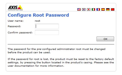
It is recommended to use the Setup Axis Camera Tool to configure the Axis Camera. If you need to configure the camera manually, follow the instructions above for connecting the camera to the computer and setting the IP, then open a web browser and enter **192.168.0.90** in the address bar and press enter. You should see a Configure Root Password page, set this password to whatever you would like, but **admin** is recommended.
